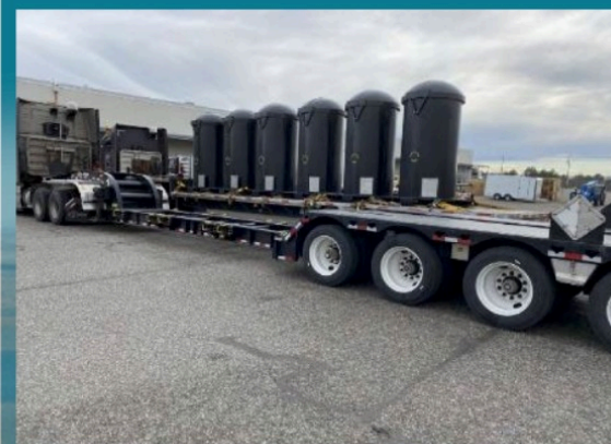
A special transporter will carry containers of vitrified waste to the Integrated Disposal Facility during direct-feed low-activity waste operations.
