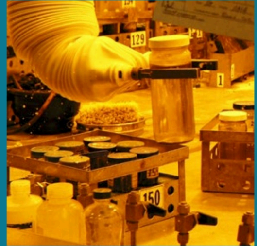
The laboratory has 11 hot cells, which allow crews to remotely handle and analyze radioactive samples.
