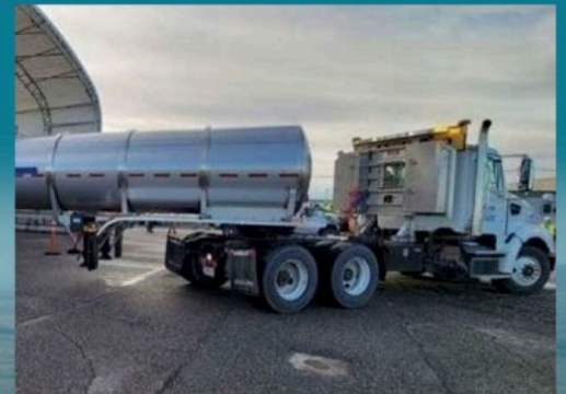
Water from the 1.2-million-gallon K West spent-fuel basin will be transported via tanker truck to Hanford's Effluent Treatment Facility for processing.
