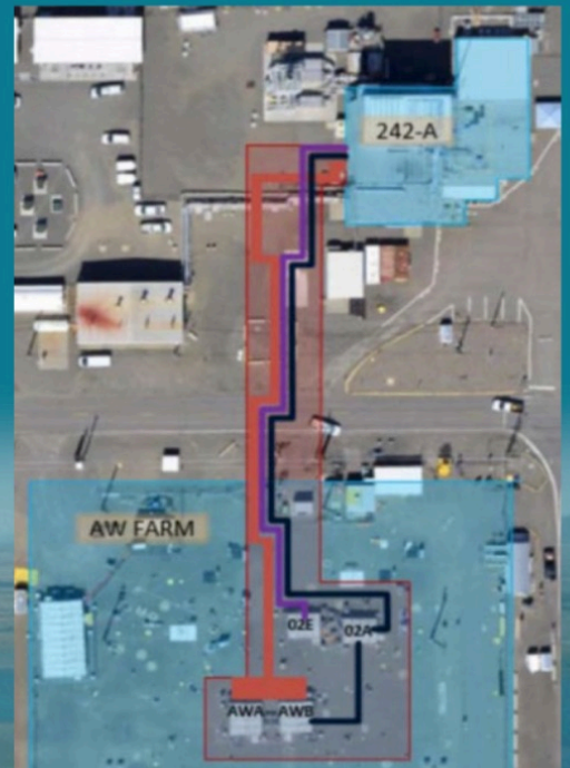
Replacement transfer lines between waste-storage tanks and the 242-A Evaporator.
