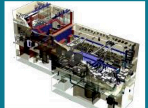
The High-Level Waste Facility contains two identical, remotely operated melter caves.
